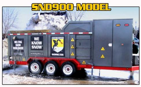
The SND900 is a 9.0 million BTU/hr machine rated at melting 30 tons of snow per hour - Based on the Latent Heat of Ice (since every manufacturer uses a different ton rating, you must compare snowmelters by their BTU's). As a result, this model is comparable to 40 Ton/hr machines being marketed to the industry.
